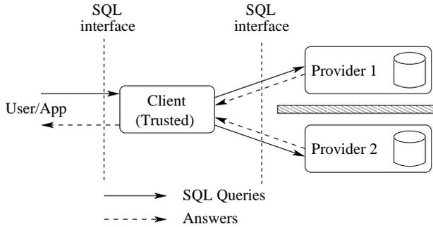
**Figure 1. Distributed Architecture for a Secure Database Service**
